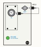
Basic configuration for testing simplex and multifiber bundles.
